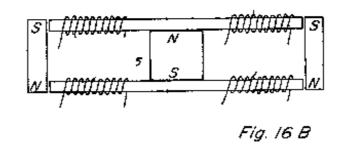
1.75 times more force is delivered to the legs of the core Than is provided by the electrical input to the control coils
